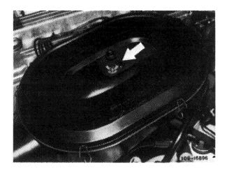
On air cleaner 2nd version the air intake proceeds directly at air cleaner, the connecting hose is no longer required.
