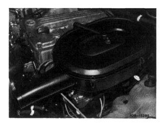
The connection for the decel shutoff valve is at air cleaner lower half.
