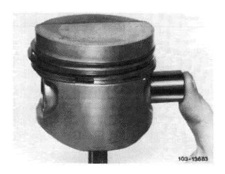
6 Place piston pin lock into groove.
