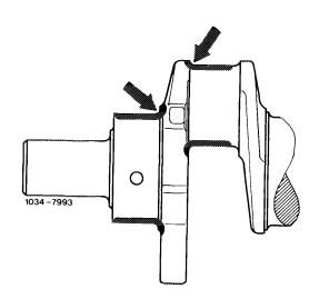
When hardening journals without hardened fillets the distance "A" between runout of hardened surface and fillet (5–6 mm) must be maintained.
