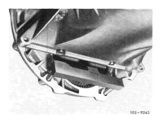
6 Unscrew bolt on crankshaft.
