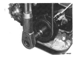
7 Mark balancing disc and crankshaft by means of a punch.
