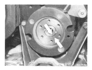
8 Pull-off balancing disc with puller.
