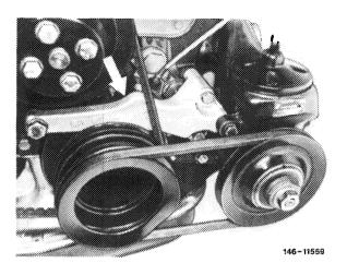
$4\,$  On model 115.015, unscrew clamp (37) of front engine stop.
