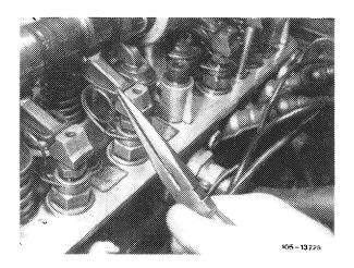
4 Push valve spring retainer down by means of pressure lever and remove rocker arm.
