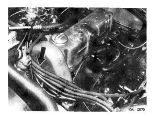
2 Set camshaft in such a manner that the rocker arm is unloaded (cam tip should point upwards).
