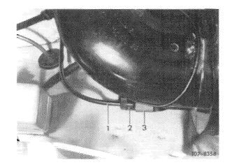
3 Loosen hex. nut (83) on idle speed shutoff valve (38) and unscrew shutoff valve.
