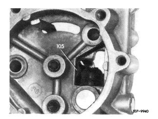
3 Check position of fast idle cam in relation to choke rod and adjust, if required.
