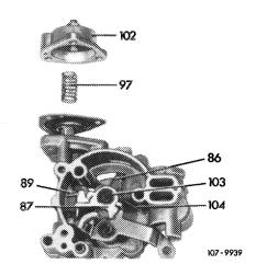
If required, install new pulldown diaphragm with diaphragm rod.
