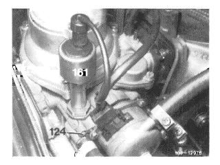
If required, pull off vacuum line on pulldown cover.
