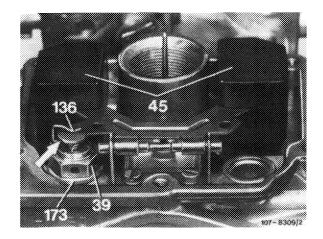
Check float level with measuring gage or slide gage at highest points of float.
