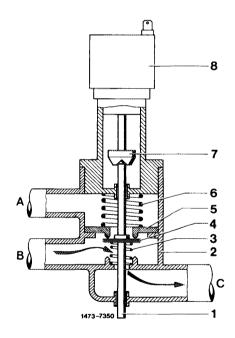
Float chamber venting system in position "external venting"
