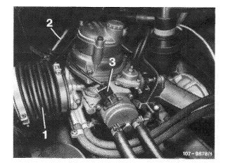
2 Remove fuel feed and return hose, as well as vacuum lines.
