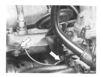
11 Plug on fuel hoses according to arrow marks on carburetor housing.
