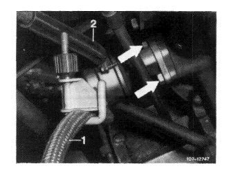
3 Rotate engine with starter motor, until vacuum value is no longer increasing. Compare indicated value with nominal value. Observe pressure drop.
