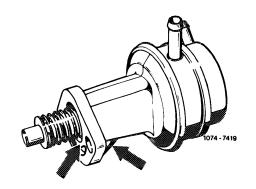
For this purpose, clean sealing surface on crankcase and coat rubber sealing ring e.g. with chalk, talcum or indian ink. Push sealing flange with rubber sealing ring against crankcase. For centering, use the two fastening bolts. Then evaluate mounting surface. If the rubber sealing ring is not resting against entire circumference, remove rubber sealing ring at crankcase end from sealing flange and install a gasket 180 091 01 80.
