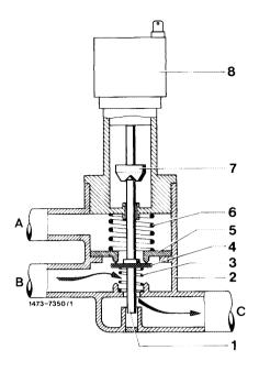
With the ignition switched on, the valve is energized. The solenoid (7) moves down and pushes the valve rod (1) in downward direction. Valve plate (4) closes connection C. The carburetor is switched to internal venting. The float chamber is now vented through bore A via valve through bore B.
