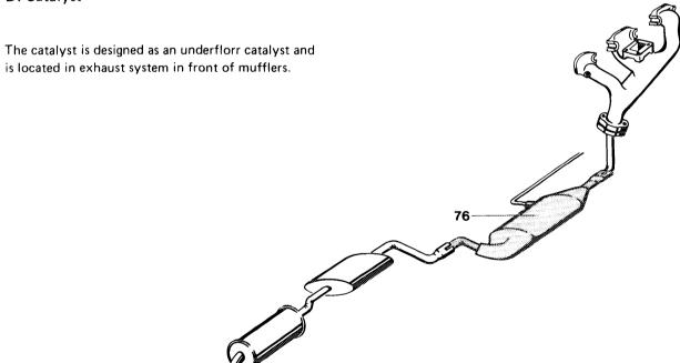
The catalyst is designed as a double bed catalyst, i.e. the housing contains two monolyths, a slim one in front and a wide one behind.
