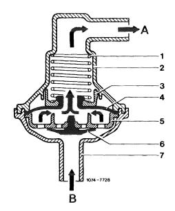
When the fuel cools down, the intake of air or fuel evaporation vapors from charcoal canister via positive vent valve (6) will compensate a vacuum of 1-16 mbar. If the vacuum in fuel tank drops below 1 mbar, the positive vent valve (6) will close.
