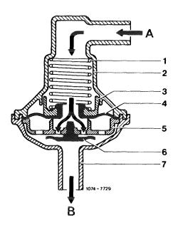
Vent valve unit open to fuel tank
