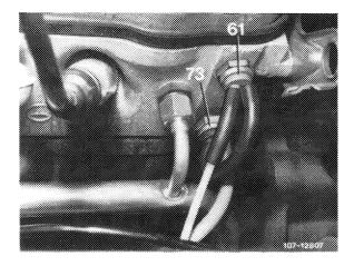
The compression spring in air switchover valve closes the injection line to cylinder head. The supplied air is injected into catalyst via check valve (42).
