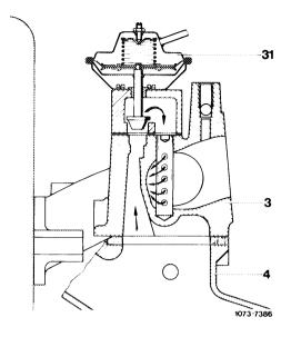
Depending on throttle valve position, the EGR valve in cylinder head is more or less supplied with exhaust gases via thermovalve 17  $^{\circ}$ C (61) in cylinder head.
