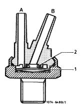
1 Bimetallic plate 2 O-ring Thermovalve 50 °C (color code black with green dot, introduced during model year 1978 color code green)
