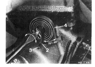
Note: On cold engine, the stop spring (2), as shown in Fig., should rest outside against stop. To make sure, and if required, slightly turn heater flap shaft away from stop to the left prior to installing stop spring.
