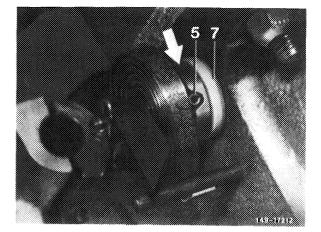
Arrow = installation position of thrust washer
