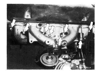
Arrows = intake manifold fastening nuts
