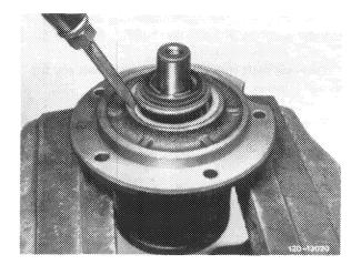
3 Force counter-ring out of impeller.
