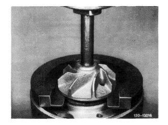
2 Apply light hammer blows at several points between bearing housing and sliding ring seal to cancel preload and force sliding ring seal out.
