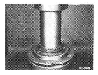
5 Coat sealing ring on counter-ring with brake cylinder paste and push with chamfered side (arrow) into thoroughly cleaned mounting bore of impeller.
