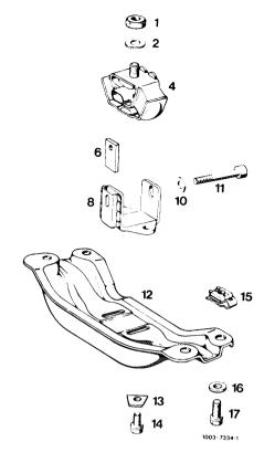
Rear engine mount with stop on vehicles with automatic transmission
