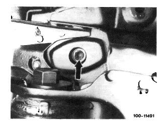
3 Lift lock (30) on front engine stop, swivel away laterally and unscrew adjusting screw (31).
