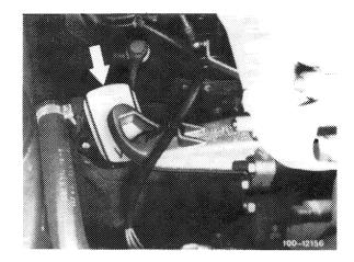
12 Position screws for engine carrier on engine mount and tighten to 70 Nm or 40 Nm.
