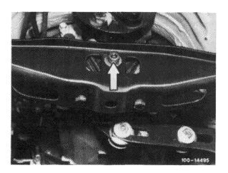
8 Lift engine with pitlift at oil pan.
