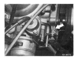
On vehicles with automatic transmission depress accelerator pedal, with engine stopped, only up to stop on kickdown switch (do not operate kickdown switch). In this position, the throttle valve lever should rest against full throttle stop (arrow) of carburetor.
