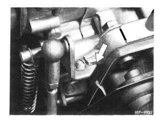
If full throttle stop is not attained, readjust Bowden wire (12) with adjusting nut (13) until throttle valve lever rests against full throttle stop.
