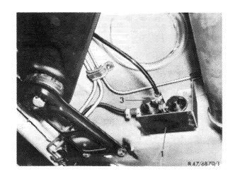
The negative vent valve (1) opens at a slight overpressure. The evaporation vapors are flowing through negative vent valve (1, direction B) into a line to engine. The line enters cylinder crankcase at pertinent connection.
