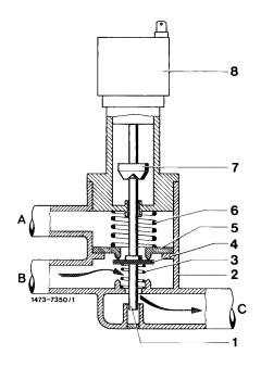
With the ignition switched on, the valve is energized. The electromagnet (7) moves downwards and pushes the valve rod (1) in downward direction. Valve plate (4) closes connection C. The carburetor is switched over to internal venting. The float chamber is now vented by bore A via valve through bore B.
