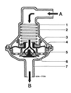
Vent valve unit open to fuel tank
