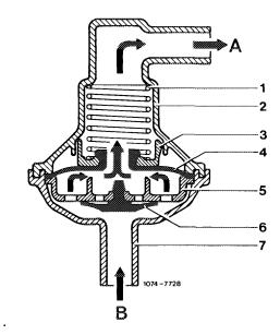
When the fuel is cooling down, the intake of air or fuel evaporation vapors from charcoal canister via positive vent valve (6) and starting at a vacuum of 1-16 mbar serves to balance the system. If the vacuum in fuel tank drops below 1 mbar, positive vent valve (6) will close.
