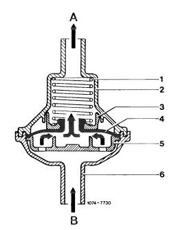
When the throttle valve is opened, the two purge holes in carburetor, which are entering a joint duct, are progressively exposed to the venturi vacuum. As a result, purging in lower partial range of engine is metered in such a manner that the driving characteristics are not influenced thereby.
