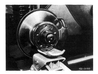
6 Check alignment with testing and adjusting pin (013b) and correct, if required. If pin points toward the center of test plate, a 0 mm deviation is indicated.
