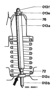
Testing and adjusting tool 013 013a Adjusting bolt
