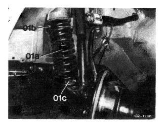
01a Tensioning screw01b Upper tensioning plate01c Lower tensioning plate
