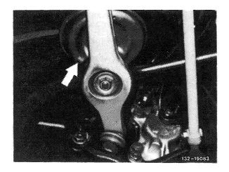
$8\,$  Tension front spring at 9 coils. Apply tensioning plates offset by  $90^\circ$
