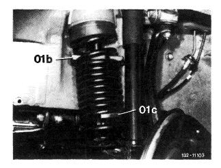
01b Upper tensioning plate 01c Lower tensioning plate
