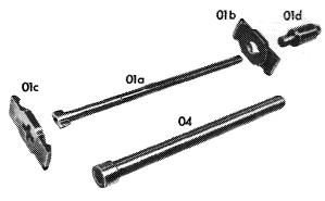
01b Upper tensioning plate 01c Lower tensioning plate 01d Guide sleeve with nut
