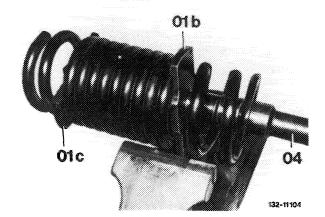
01b Upper tensioning plate01c Lower tensioning plate04 Socket
