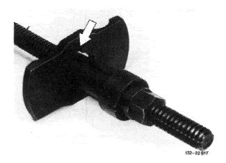
5 Tension front spring while lifting lower control arm by means of the vehicle jack to facilitate tensioning.
