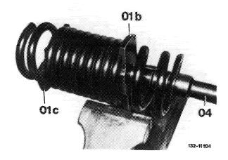
9 Place rubber mount on front spring with a screwing motion.
