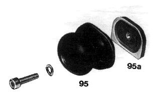
95 Auxiliary rubber spring 95a Spacing washer
