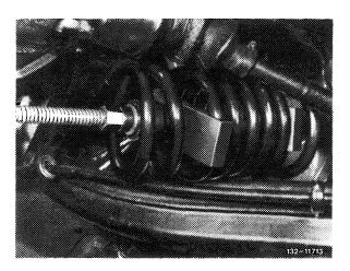
7 Clamp upper tensioning plate and slacken rear spring.
