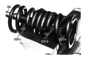
020a Tensioning screw 020b Upper tensioning plate 020c Lower tensioning plate 04 Socket
