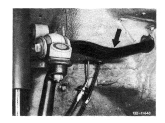
11 Mount support of upper control arm torsion bar.
