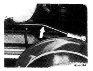
9 Mount locking plates (82a) and attach tosion bar with holding brackets (82) left and right to frame floor.
