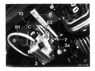
2 Loosen connecting rod left and right on torsion bar (arrow).
