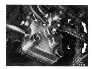
10 Evacuate basic pressure via bleed screw (038n) and oil drain hose (061). Unscrew pressure tester (038), screw bleed screw into level controller.
