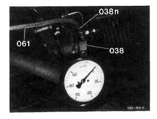
5 To check pressure oil pump and pressure relief valve in level controller, push lever of level controller into position "F" (filling). Keep engine running and watch pressure gauge.
