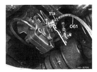
4 Connect pressure tester (038) to level controller or to distributor. Plug oil drain hose (061) on bleed screw (038n).
