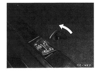
4 Remove cover for frame cross member after loosening the five Phillips head sheet metal screws (arrows).
