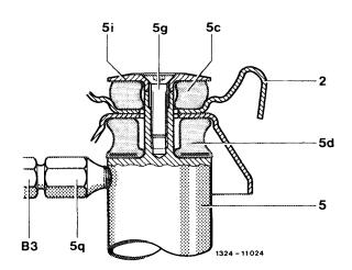
19 Tighten screw connection and pressure hose, while paying attention to correct position of hose. If required, change position of hose on ring fitting of pressure reservoir.
