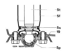
7 Tighten ball joint to specified tightening torque with special tool (04,05).
