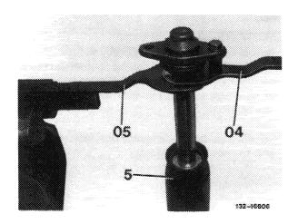
4 Connect pin spanner (04) with fastening eye of ball joint and loosen ball joint.
