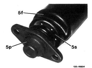
5f Dust guard 5p Ball joint 5s Disc
