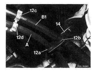
7 Connect and install oil connection hose on suction line (A).
