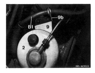
**Note:** On vehicles with automatic climate control, remove oil supply tank.
