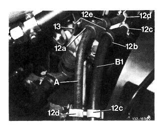
8 Connect HP expansion hose (B1) and install.
