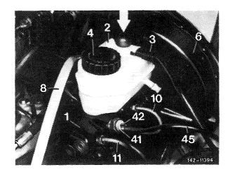
5 Loosen tandem main cylinder on brake unit and remove, while paying attention to O-ring located in groove of tandem main cylinder flange.
