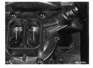
Layout of plate valves in system circuit B. Cover with screw connection.
