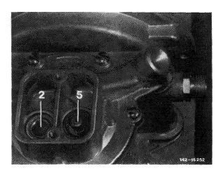
Layout of plate valves in system circuit K. Cover without screw connection.
