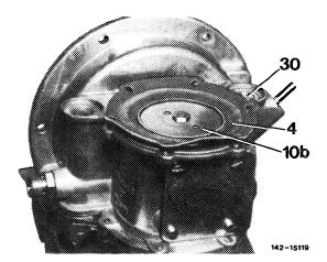
8 Upon installation of check valve (30), place new sealing rings (24) into pump housing.
