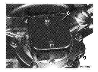
3 Remove both compression springs (32), plate valves (2 and 5) and the two sealing rings. Unscrew slotted screws from pump cover (9) and remove pump cover. Clean pump cover.
