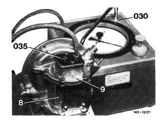
11 Push pump cover (9) against housing (8) at spots designated by arrows. Use hand pump in tester (030) to establish a vacuum of min. 0.5 bar. If vacuum remains constant without actuating hand pump, tighten slotted screws in pump cover to specified torque of 5 Nm.
