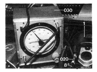
Note: The measuring connection is self-made according to specified dimensions (parts 1, 3, 4, 5 and 6 are brazed to each other). For connection to brake booster the pipe section and coupling nut of an old vacuum line may be used. Connection to vacuum line is made by means of a screw connection.
