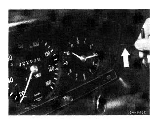
3 Engage at recess (arrow) and pull out slightly.
