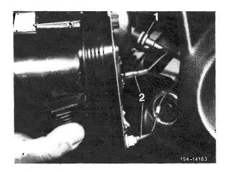
6 Disconnect line for oil pressure gauge (1), (apply counterhold with 2nd open-end wrench and remove instrument cluster toward the right).
