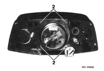
3 Slightly cant tachometer and remove toward the right.
