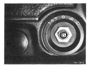
5 Remove rotary light switch from instrument panel in downward direction.
