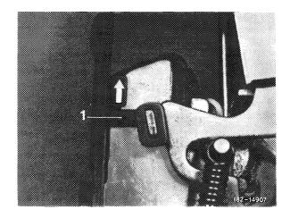
Slide backdoor contact switch on removed backdoor lock in direction of arrow, slightly pushing down detent cam (1).
