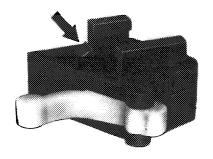
Removed backdoor contact switch
