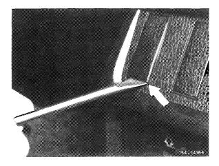
2 Remove switch of heatable rear window.
