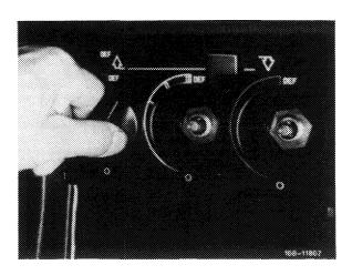
7 Unscrew nuts on control unit (wrench size 24 mm).
