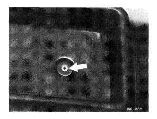
14 Lift rear of center console and pull it out of instrument panel. Prevent front end of center console from spreading apart.
