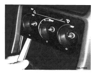
11 Unscrew bolts on both sides of front tunnel section.
