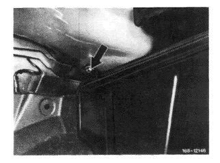
2 Remove both bottom screws from trunk floor plate and take out partition.
