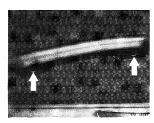
8 Unclip door cover at the side and bottom from the door inner panel. Offer plastic wedge as close as possible to clips.
