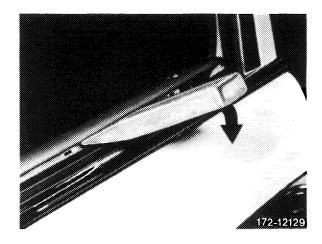
7 Lift front of door liner far enough that the hook can be lifted out of inside door panel.
