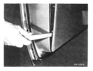
**Note:** Two clips at the top **front** and one clip at the bottom must be unclipped.
