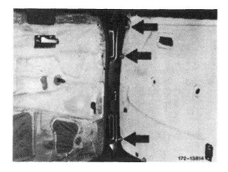
9 Starting at the rear, lift door cover out of the upper retaining clips, and, while doing so, insert plastic wedge between locking lever and door cover.
