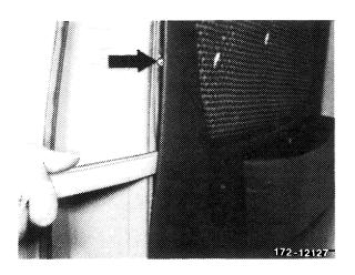
6 Pry door liner off of upper clips with a plastic wedge.
