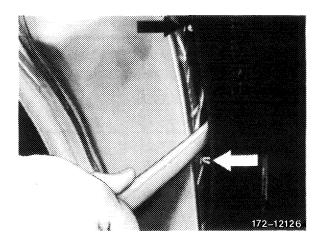
8 Insert hand between door liner and inside door panel, and press out the clip (arrow) in area of ashtray.
