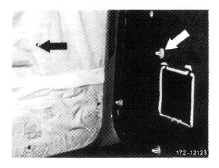
9 Press door liner off of top clips with a plastic wedge.
