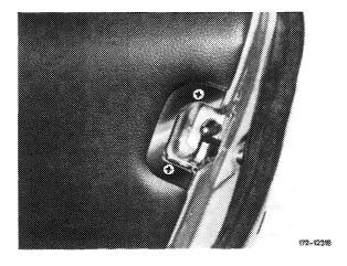
5 Press bottom retaining cam on ashtray housing out of door liner.
