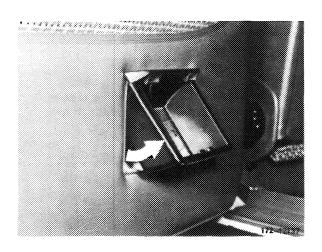
7 Unclip side and bottom of door liner at inside door panel. Insert plastic wedge as close to clips as possible.
