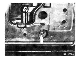
10 Pull out guide rail at the top of the door shell. To do so, it is necessary to turn the guide rail by 90° so that the thread stud welded to the lower part does not impair removal.
