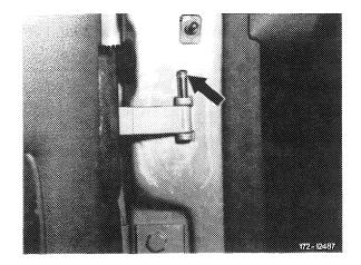
2 Use a plastic wedge to press clips on front side of door (along with retaining rail for front door) off of door panel.
