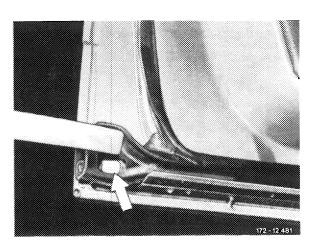
4 Pull rubber frame out of door seam and remove.
