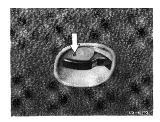
4 Slip welding wire with hook through tapped hole for upper fastening screw and attach to release lever. Pull back release lever with welding wire so that the trigger foot can snap back to its starting position.
