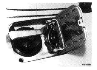
2 Unscrew both screws and remove tank flap.
