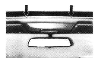
3 Remove left and right sliding rails.
