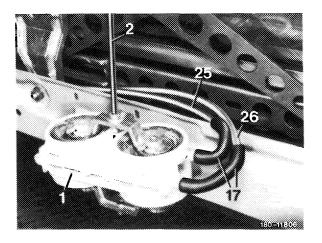
6 Loosen lock washer (43) of shift rod (2) on vacuum element (1) and pull out shift rod.
