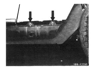
**Note:** A tripod radiator, a large welding burner with a long soft flame or a hot air blower (600 °C) may be used. With proper care, the fender can be heated without damaging the paintwork. Damaged fenders which are not used any longer, can be heated faster from above on surface.
