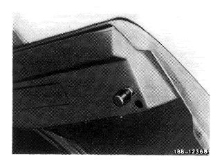
30 On vehicles with inner fender, introduce repair preservation of cavity through opening in wheelhouse.
