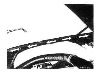
18 Lift front fender, starting at the front and pull out in forward direction.
