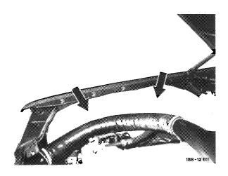
15 Lightly heat contact surface of fender in headlamp housing and loosen in this range first.
