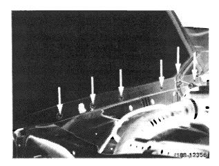
10 Remove screws on front wall pillar by means of an articulated wrench.
